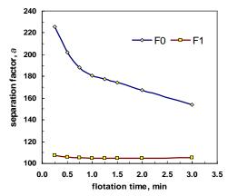
Fig. 5. Results of laboratory batch tests on reflotation of final industrial copper concentrates performed in the absence (F0) and presence (F1) of dextrin, shown as Cu content in the froth
