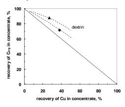
Fig. 4. The Fuerstenau upgrading curve showing relation between recovery of C<sub>org</sub> in the cell product and Cu recovery in the froth product for industrial trial of reflotation in the absence and presence of maltodextrin DE 6-8 at the dose of 1.93 kg/Mg. The throughput was 7640 Mg per shift, concentrate yield 6,84%
