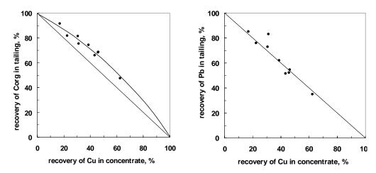
Fig. 3. Results of reagent free reflotation of the final industrial flotation copper concentrates leading to different Cu and Corg recoveries in the two products of the process at ZWR Rudna (O/ZWR, 2010, series I). Reflotation performed with industrial flotation machines MF011 and MF013. Different data points were obtained by varying flotation conditions. Separation results from different kinetics of Cu and Corg flotation (Fig. a). No separation between Cu and Pb is observed (Fig. b)
