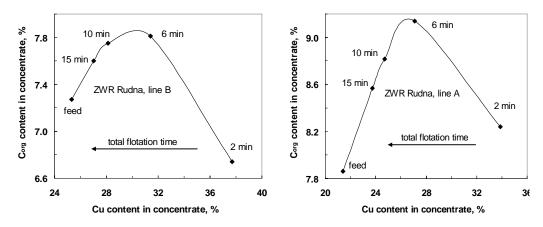
Fig. 2. Relation between organic carbon and copper content in the refloated in a laboratory flotation machine final industrial copper concentrate from side A and side B of ZWR Rudna (O/ZWR, 2009)
